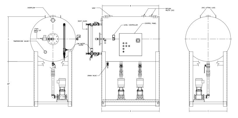
A surge tank increases the storage capacity of boiler feed system. It performs similar function to a boiler feed unit except it feeds a deaerator instead of a boiler. A surge tank is typically used on systems having more than 20% hot condensate returns.
